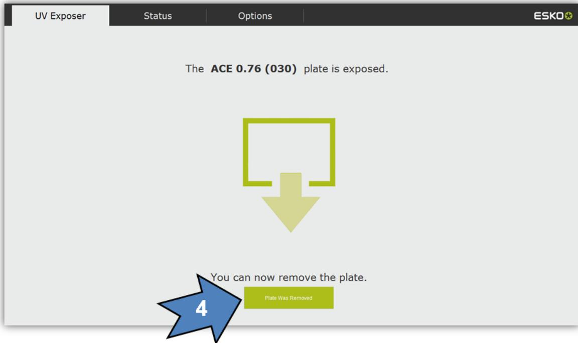
The end of the exposure is shown. The removal of the plate from the XPS Crystal must be confirmed (4).
